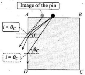
When angle of incidence on AD of the ray emanating from pins is greater than the critical angle, the light suffers from total internal reflection and cannot be seen through AD.
