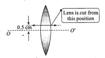
The top part is placed at (0, 0) and an object placed at (-50 cm, 0). There is no effect on the focal length of the lens.
