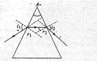
According to Snell's law,  $1 \cdot \sin i_1 = \mu \cdot \sin r_1 \Rightarrow i_1 = \mu \cdot r_1$
