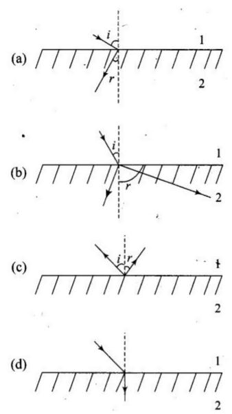
**Solution:** (a) The materials with negative refractive index responds to Snell's law just opposite way. If incident ray from air (Medium 1) incident on those material, the ray refract or bend same side of the normal as in option (a).
