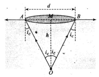
Rays of light incident at an angle greater than  $i_{\rm C}$ , are totally reflected within water and consequently cannot emerge out of the water surface.
