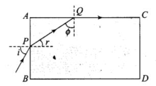
Any ray is guided along AC if the angle ray makes with the face AC ( $\phi$ ) is greater than the critical angle. From figure
