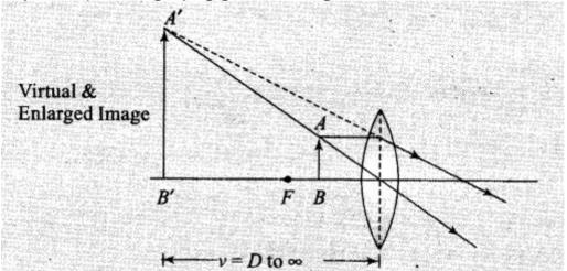
For magnification when final image is formed at D and  $\infty$  (i.e.,  $m_D$  and  $m_{\infty}$ ).
