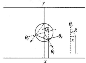
Here the material has refractive index -1,  $\theta_r$  is negative and  $\theta'_r$  positive.
