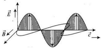
The direction of propagation of electromagnetic wave is perpendicular to both electric field vector  $(\vec{E})$  and  $\vec{B}$  magnetic field vector B, i.e., in the direction of  $\vec{E} \times \vec{B}$ .
