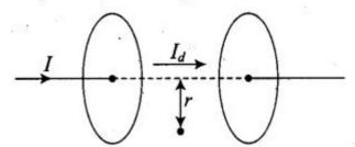
The magnetic field at a point between two plates of capacitor at a perpendicular distance r from the axis of plates is given by
