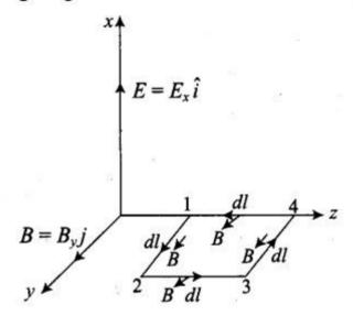
$$\oint \vec{B} \cdot d\vec{l} = \int_{1}^{2} \vec{B} \cdot d\vec{l} + \int_{2}^{3} \vec{B} \cdot d\vec{l} + \int_{3}^{4} \vec{B} \cdot d\vec{l} + \int_{4}^{1} \vec{B} \cdot d\vec{l}$$
