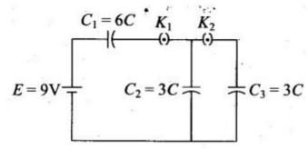
**Solution:** In the circuit, when initially  $K_1$  is closed and  $K_2$  is open, the capacitors  $C_1$  and  $C_2$  connected in series with battery acquire equal charge.
