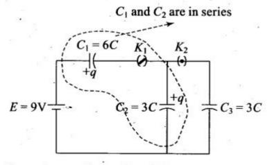
Hence the charge in capacitors  $C_1$  and  $C_2$  are
