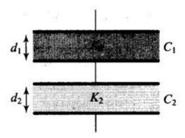
$$\frac{1}{C_{\text{eq}}} = \frac{1}{C_1} + \frac{1}{C_2} \Rightarrow C_{\text{eq}} = \frac{C_1 C_2}{C_1 + C_2}$$
