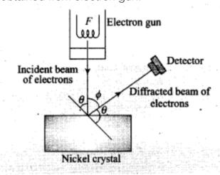
2. The diffracted beam of electrons is received by the detector which can be positioned at any angle by rotating it about the point of incidence. The energy of the incideni beam of electrons can also be varied by changing the applied voltage to the electron gun.
