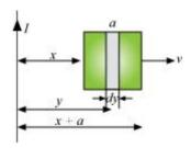
Magnetic flux associated with element dy,  $d\phi = BdA$
