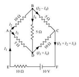
I<sub>1</sub> = Current flowing through the outer circuit
