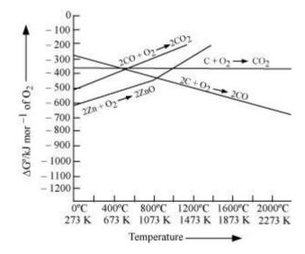
Reduction of ZnO to Zn is usually carried out at 1673 K. From the above figure, it can be observed that above 1073 K, the Gibbs free energy of formation of CO from C and above 1273 K, the Gibbs free energy of formation of  $CO_2$  from C is lesser than the Gibbs free energy of formation of ZnO. Therefore, C can easily reduce ZnO to Zn.
