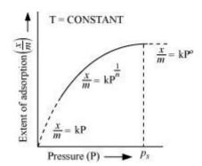
The plot between the extent of adsorption  $\frac{m}{m}$  against the pressure of gas (P) at constant temperature (T) is called the adsorption isotherm.
